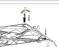
3. Install the Fan module on the PCI slot by Screw B.
