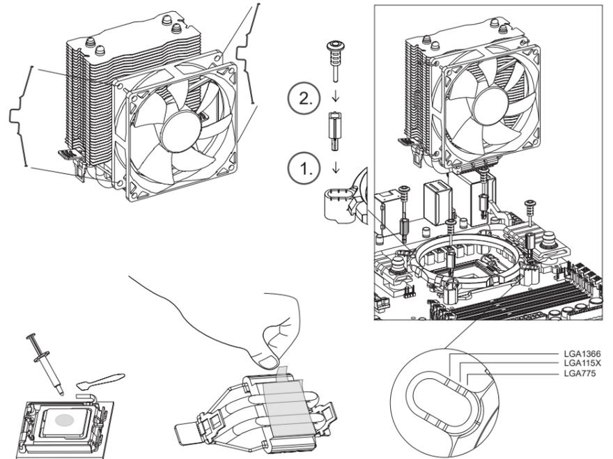
1. Mount the 92mm Fan (A) by inserting the Fan Mount Set (D) into the fan mounting holes and fastening in Heatsink (B) grooves.
