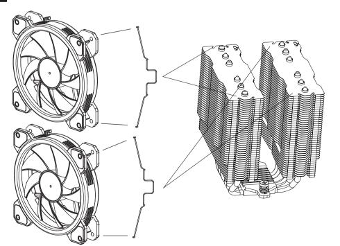
9. Mount 2 x 120mm Fan by inserting 2 x Fan Mount Set L into the fan mounting holes and
