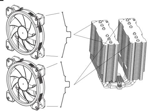
8. Mount 2 x 120mm Fan by inserting 2 x Fan Mount Set L into the fan mounting holes and buckling in heatsink grooves.
