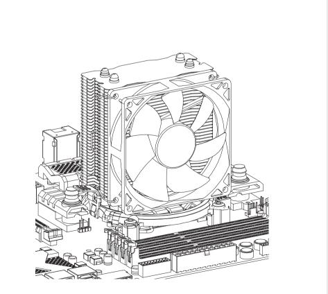
1. Mount the 92mm Fan (A) by inserting the Fan Mount Set (D) into the fan mounting holes and fastening in Heatsink (B) grooves.
