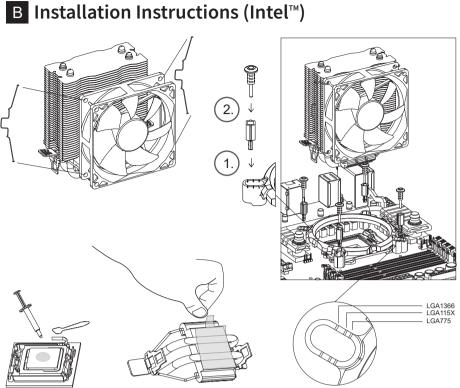
1. Mount the 92mm Fan (A) by inserting the Fan Mount Set (D) into the fan mounting holes and fastening in Heatsink (B) grooves.
